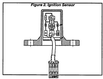
See Figure 3. The Sensor circuit board mounts solid state components which are sensitive to magnetism. Magnets in the Ignition Cage rotate past the Sensor, causing the base of a transistor to be "pulsed". The transistor acts much like a "switch" or a set of "contact points". Pulsing the transistor base causes the "switch" to close and connect the "OUT" lead to the "GND" lead. This triggers the Ignition Module to deliver a primary Ignition current to the Ignition Coil at timed intervals.
